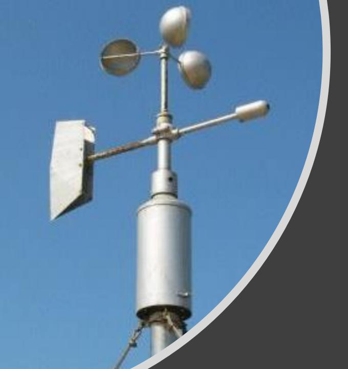
The anemometer was invented in 1845 in Ireland for the purpose of measuring the speed of the wind.
