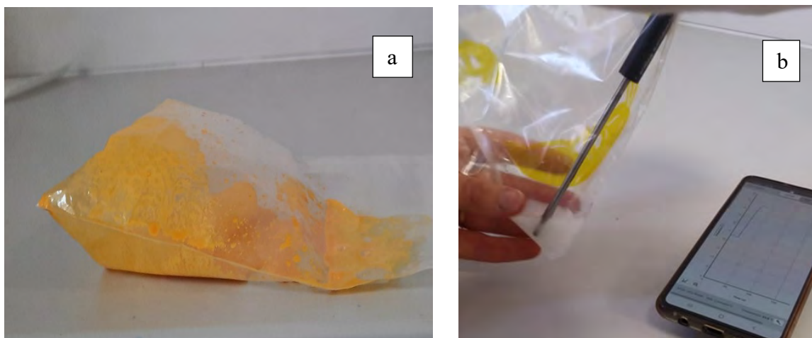
Figure 2: Baggy experiment investigations. (a) showing colour change and inflation of bag; (b) measuring temperature change of \text{CaCl}_2 with water.
