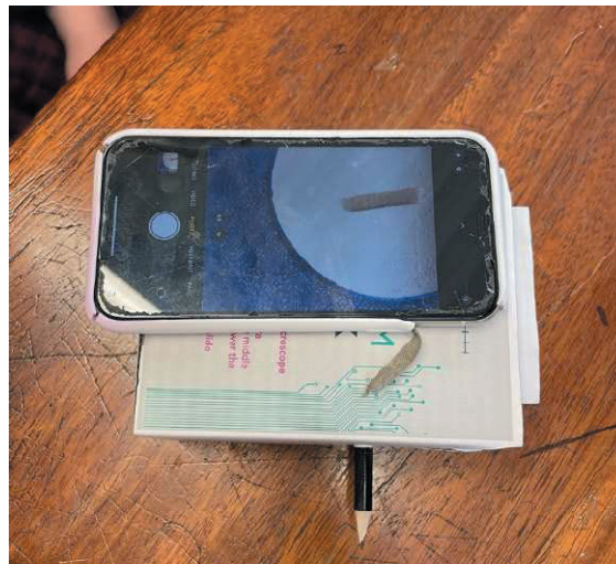
Student-constructed microscope using their cell phone camera
