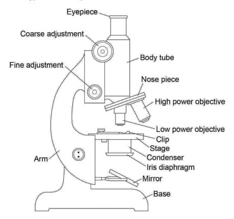
Some microscopes have a built-in light instead of a mirror.
